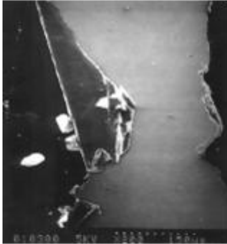
Figure 2. 16 Delamination from copper CMP
